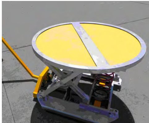
Fig 2.1.22: Adjustable height turntable
